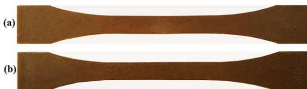
Scheme 1. Profile of the wood flour/PLA composites. (a) without MA; (b) with MA. [Color figure can be viewed in the online issue, which is available at wileyonlinelibrary.com .]
